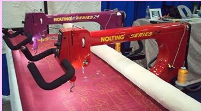
The NV Machine is the newest in the fleet of Nolting machines. This machine has a touch screen with programmable stitch regulation. You can stitch in 4 different stitch modes plus single stitch and needle up/down. It also has an adjustable brightness LED work light. This machine can also be equipped with a computer.
