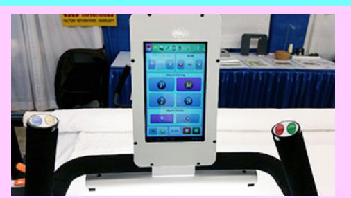
mmable stitch regulation. You can stitch in 4 different stitch modes plus single stitch and needleup/down. It also has an adjustable brightness LED work light. This machine can also be equipped with a computer.
