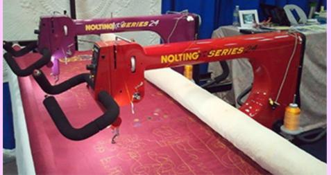
handles in the front & rear. The Pro Machine comes in 20", 24" and 30" reach with 10-12" of inside height. There are easy dials on the front to set stitch length and other options. This machine can also be equipped with a computer.
